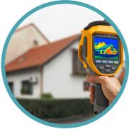
It is a critical tool used by designers to eliminate thermal bridging, a significant cause of energy loss.
